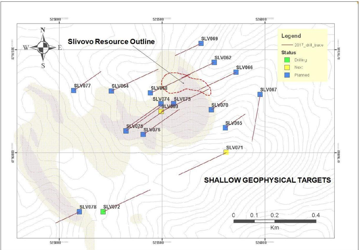
**Figure 2.** Phase 1 drill plan showing SLV062, 063, 064, 066, 068, and 069 targeting the Main Gossan Offset; SLV065, 067, and 070 targeting the SE Gossan Extension; SLV073, 074, 075, and 076 targeting the Sandstone Gossan; and SLV077 targeting the Buena Oro zone.
